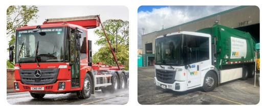
Typically branded as Freightliner in the US, the Mercedes/Daimler Econic is a best-inclass direct vision truck currently in use in the US. Available as all electric or with a conventional engine, the Econic was developed specifically
