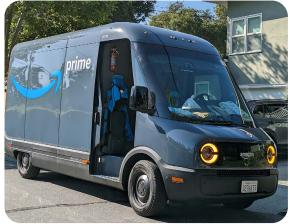
The low-entry/cab-thru design of the new Amazon Rivian van makes it easier for drivers to get in and out of the vehicle safely. Image: Mliu92.
