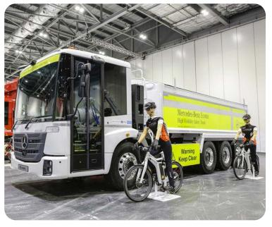
The "bus-style" passenger side door increases driver visibility. Image: Torque.
