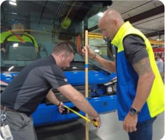
Measuring front visibility with TSR's 5-Star Rating System. Image: TSR.
