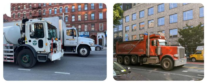
Window placement, cab height, and hood size and shape all directly impact driver visibility. The driver in the DSNY Sanitation truck (front left), can see the road better than the driver of truck next to them, and can see the road significantly better than the driver of the orange truck (right). Images: Kate Fillin-Yeh.
