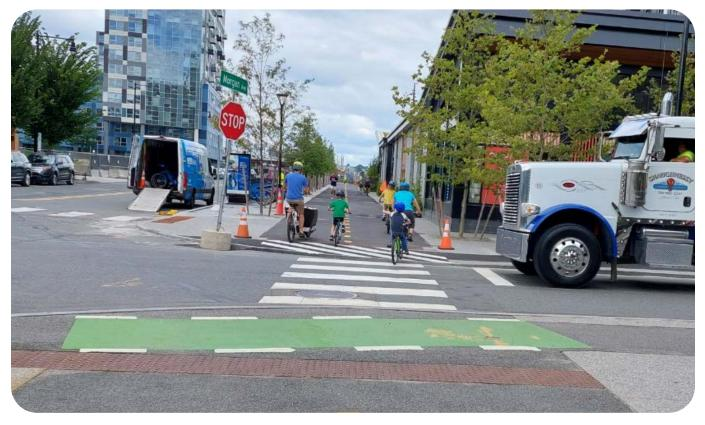
A conventional truck in Cambridge, MA. The design of this truck cab means that, even though the driver has stopped appropriately at the stop bar, they cannot see the people or cyclists in the crosswalk directly in front of them. Image: Alexander Epstein.
