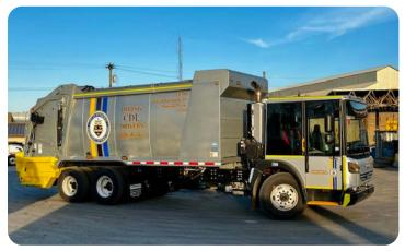
The Dennis-Eagle ProView is a best-inclass direct vision truck currently in use in the US. It features low-entry, walk-thru with a variety of driver comfort features such as noise-reduction, and significant vision improvements to the front and side. Some models include a "bus-style" passengerside door which increases side visibility even further. Notably, the ProView is in use in Pittsburgh, PA as a staple of its sanitation
