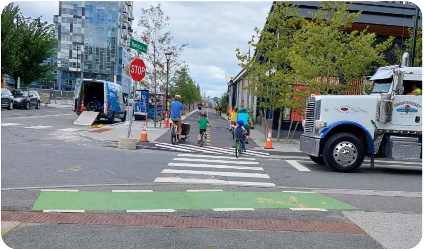
A conventional truck in Cambridge, MA. The design of this truck cab means that, even though the driver has stopped appropriately at the stop bar, they cannot see the people or cyclists in the crosswalk directly in front of them. Image: Alexander Epstein.
