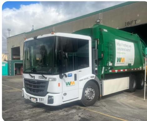
Typically branded as Freightliner in the US, the Mercedes/Daimler Eonic is a best-in-class direct vision truck currently in use in the US. Available as all electric or with a conventional engine, the Eonic was developed specifically
