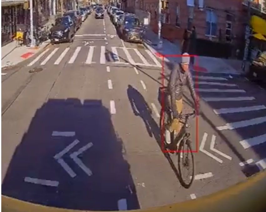
Figure 1. Image from VisionTrack system (left). Drivers also saw a warning icon when the VRU was detected (right).
